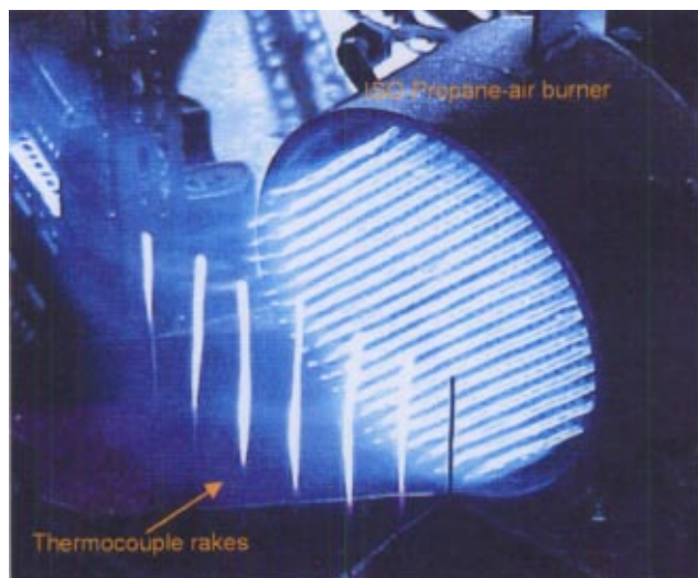
Fig. 2 ISO burner temperature calibrations
