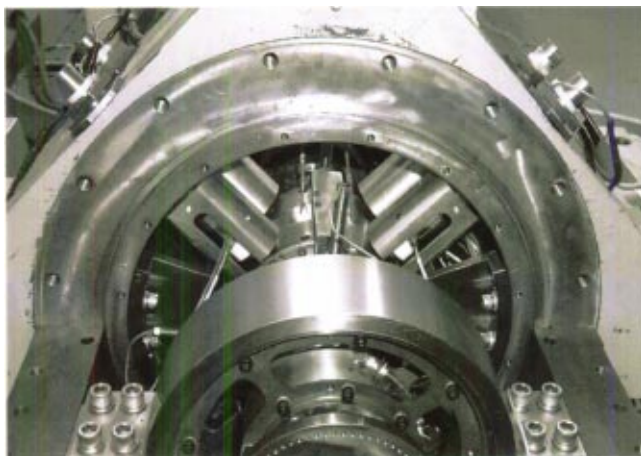
Fig. 11 Load measurements at the stator using piezoelectric actuators
