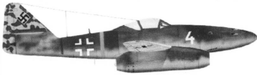
Fig. 12 The Me-262 powered by two Junker Jumo 004B turbo-jets. Dr. Bentele was instrumental in resolving a major operational blade vibration problem with this engine.
