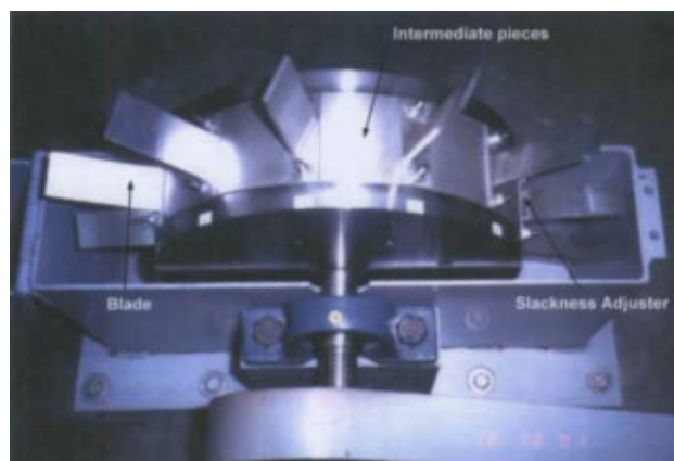
Fig. 4 Photograph showing blade assembly with intermediate locking pieces
